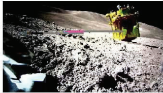
Japan's SLIM moon lander, including battery, survived three freeze-thaw cycles on the lunar surface
