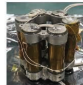
Soft Li-ion cell and CADRE lunar rover battery modules
