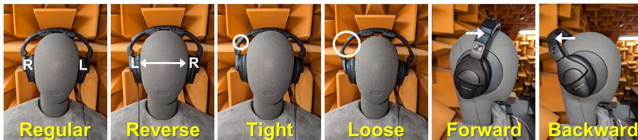
Figure 3. Six headphone configurations used to examine measurement variability.
