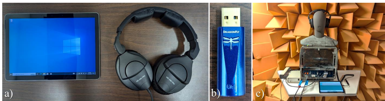
Figure 1. a) Microsoft Surface Go 3 tablet computer and a pair of Sennheiser HD 280 headphones, b) DragonFly Cobalt USB DAC, and c) HEAD Measurement System with the psychoacoustic testing kiosk in a small anechoic chamber.
