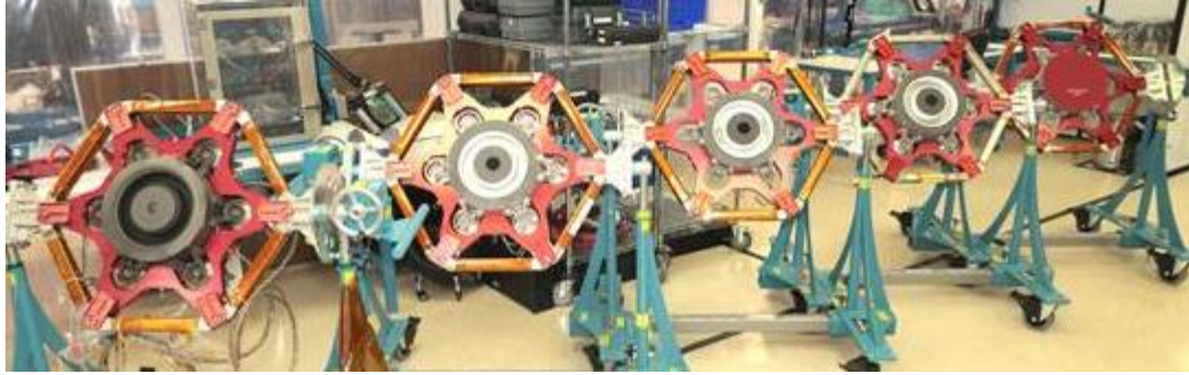
Figure 4: AEPS Qualification and Flight Thrusters at Aerojet Rocketdyne, Redmond WA prior to acceptance testing of Flight 1
