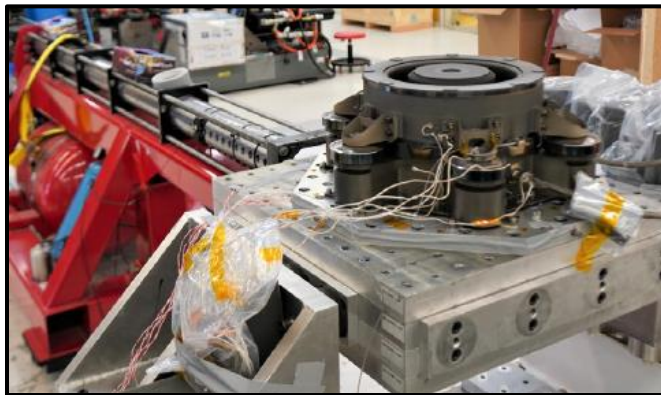
Figure 15: QM1 during shock testing at Moog, CSA in Mountain View, CA
