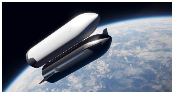
Figure 13. Artist's illustration of the on-orbit cryogenic propellant transfer between SpaceX Depot (white) and Tanker (gray). (Image credit: SpaceX)
