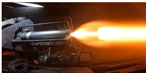
Figure 11. In 2025, NASA Marshall tested a hybrid motor for an upcoming PSI test in NASA Langley's 18.2 m (60 foot) spherical vacuum chamber.
