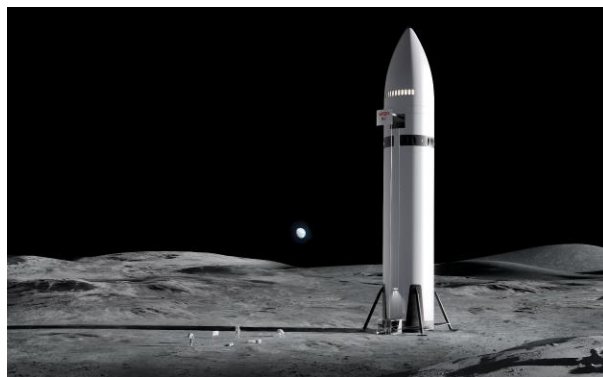
Figure 3. SpaceX is contracted to provide Starship HLS lunar lander capable of supporting two crew members for a 6.5-day surface expedition during Artemis III. (Image credit: SpaceX)
