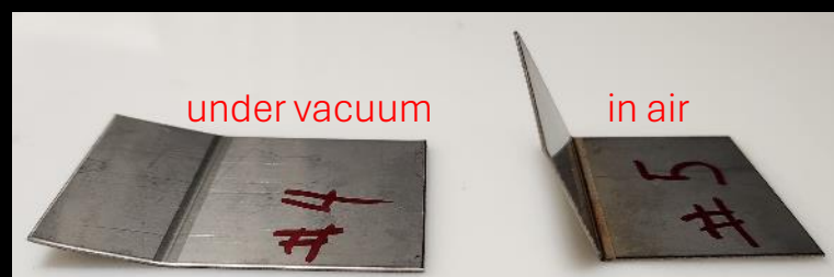
Laser bent AISI 304 stainless steel, 0.6 mm thick
