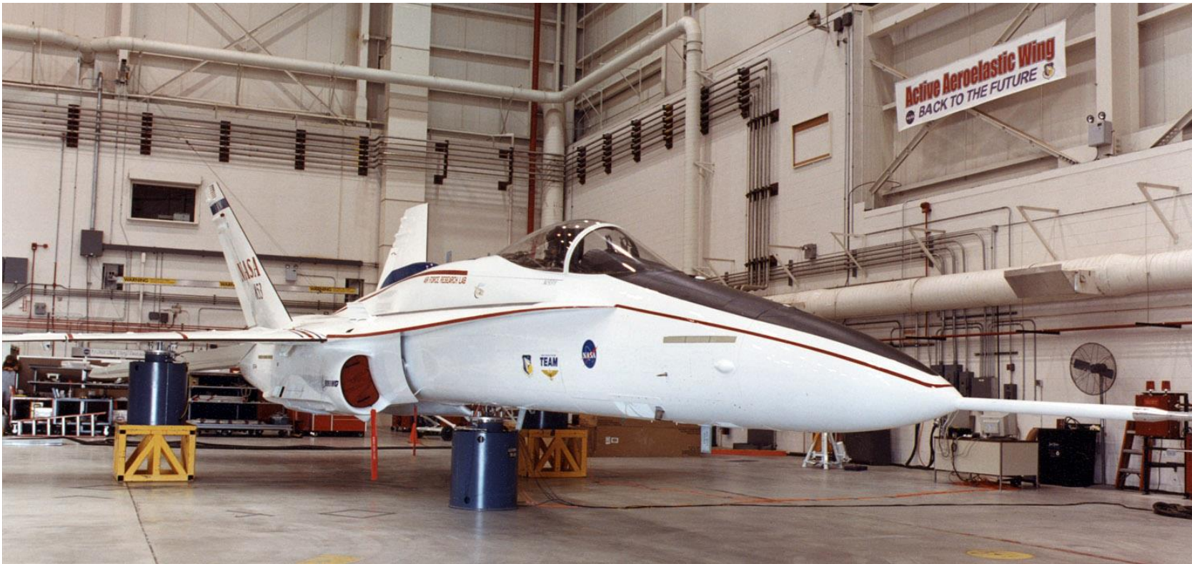
F-18, Active Aeroelastic Wing (AAW) on Soft Supports BEFORE Self-Jacking System
