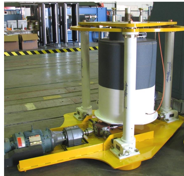
60K3S, One Self-Jacking Canister Holds 20K lbs
