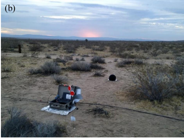
FIG. 1. The microphone array deployed by BYU during the CarpetDIEM test campaign. (a) The microphone locations, indicating the two different microphone types deployed. (b) A photograph of the data acquisition unit and the center microphone.
