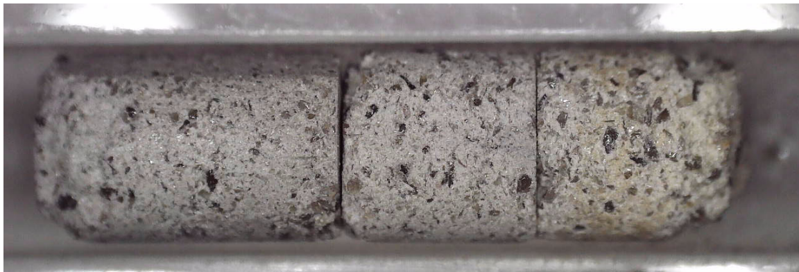
Final pellets after the run to 1000C in UHP argon on 5M Glass pellets from Matt Creedon
