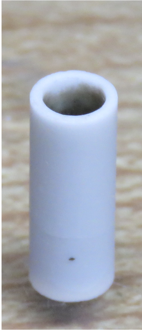
(left) Crucible with test sample after run ,
