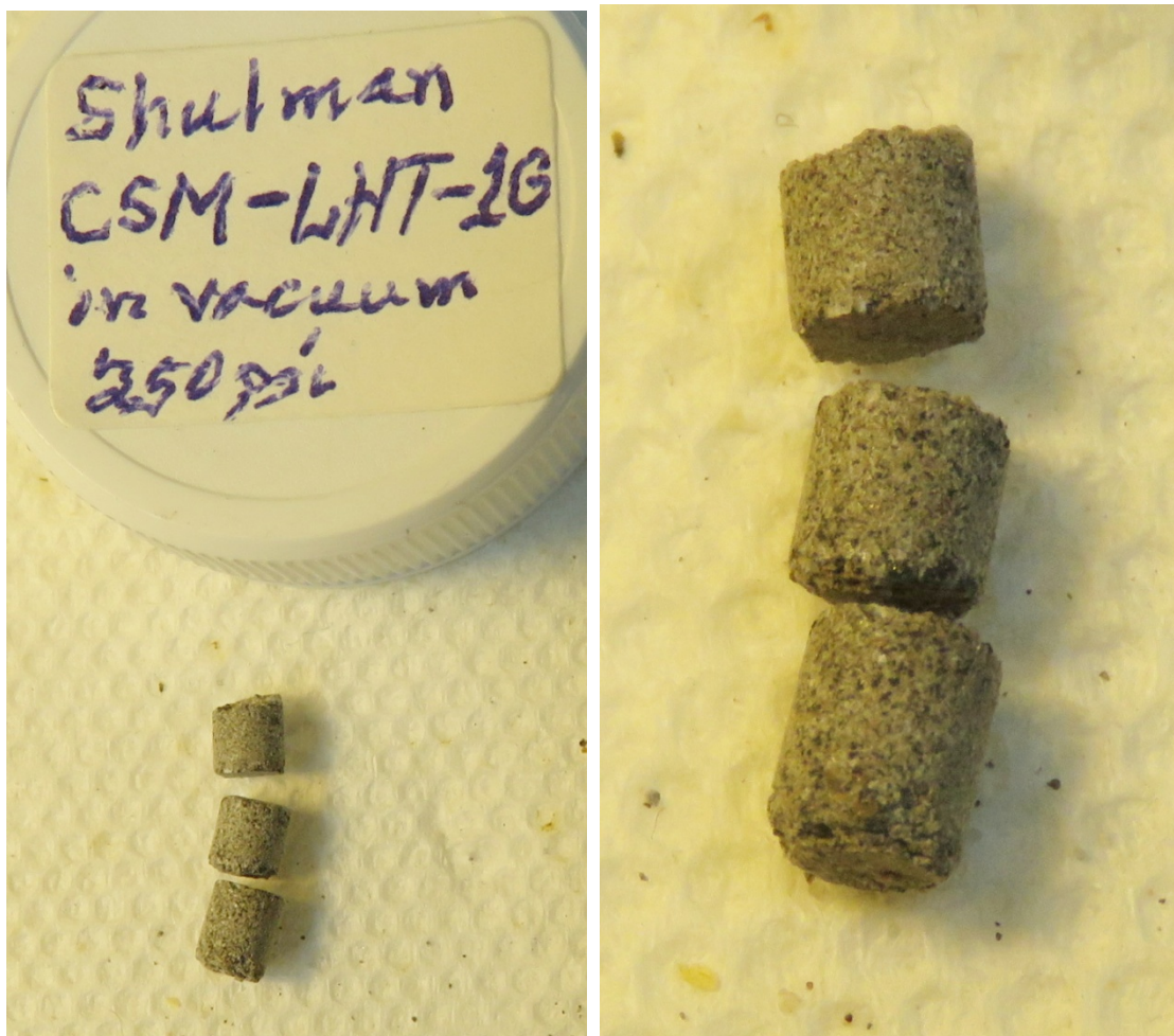
Final pellets after the cycle to 1100 C in vacuum ( at a pressure of less than 1 milliTorr ).
