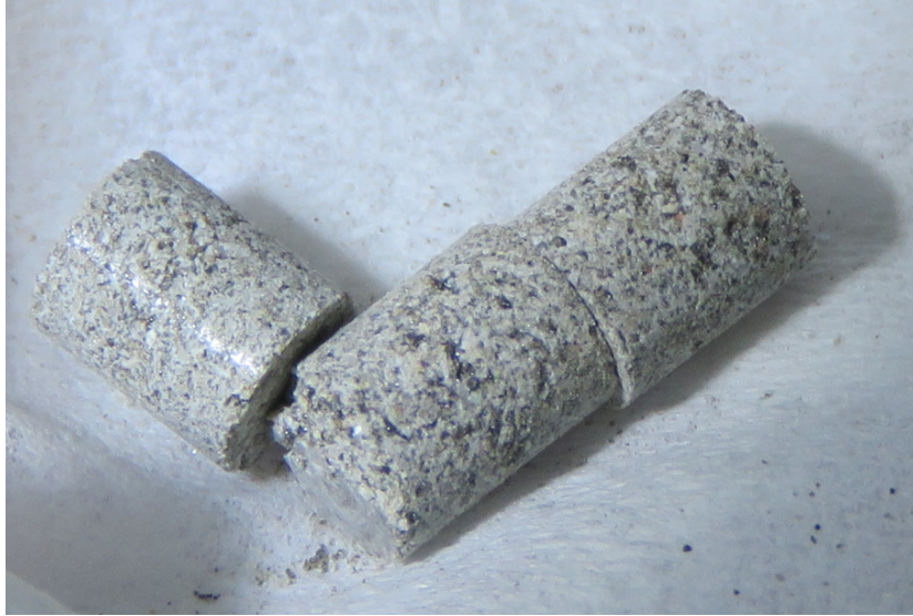
Three initial pellets after baking at 200 C in air.
