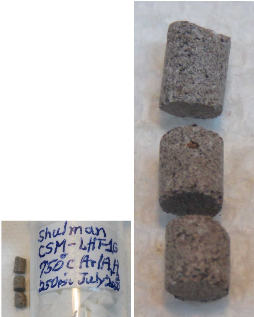
Final pellets after the cycle to 1100 C in vacuum ( at a pressure of less than 1 milliTorr ).
