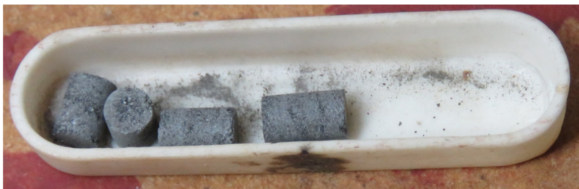
Initial Pellets after pressing – 4 pellets
