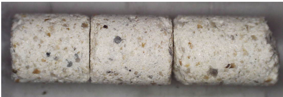
Three final NUW-LHT-5M stimulant pellets after a cycle to 1150C in UHP argon .
