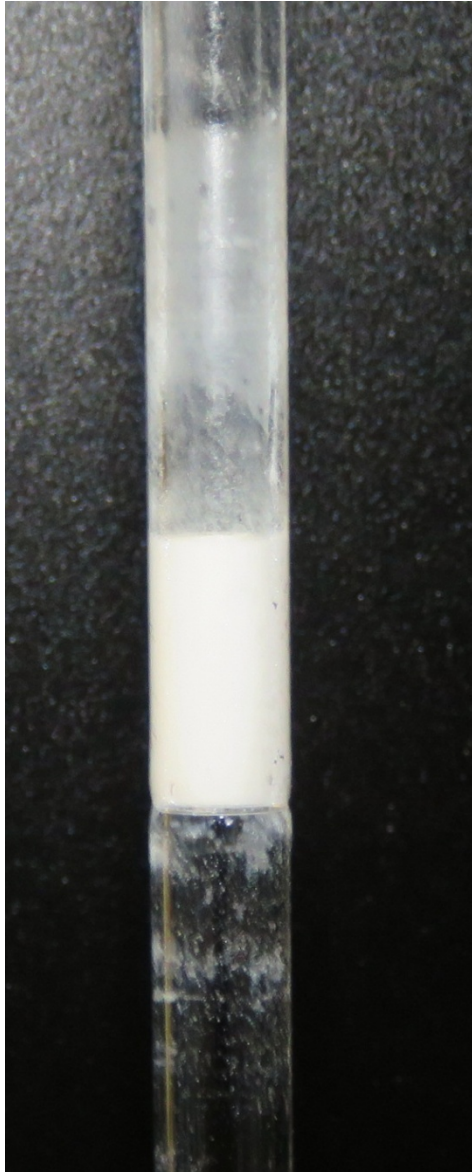
( left) Alumina crucible in holder after cycle to 1400 C in 10 sccm flowing UHP argon. (right) Holder with crucible and fused silica “plug” ,before insertion of test pellets .
