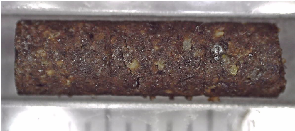
Final sample, after cycle to 1250 C in UHP argon.
