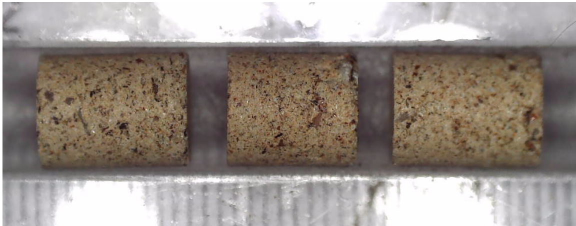
Three final NUW-LHT-5M pellets after a cycle to 1150C in UHP argon .
