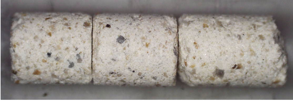
Three final 5M Glass pellets after the cycle to 1150C in UHP argon
