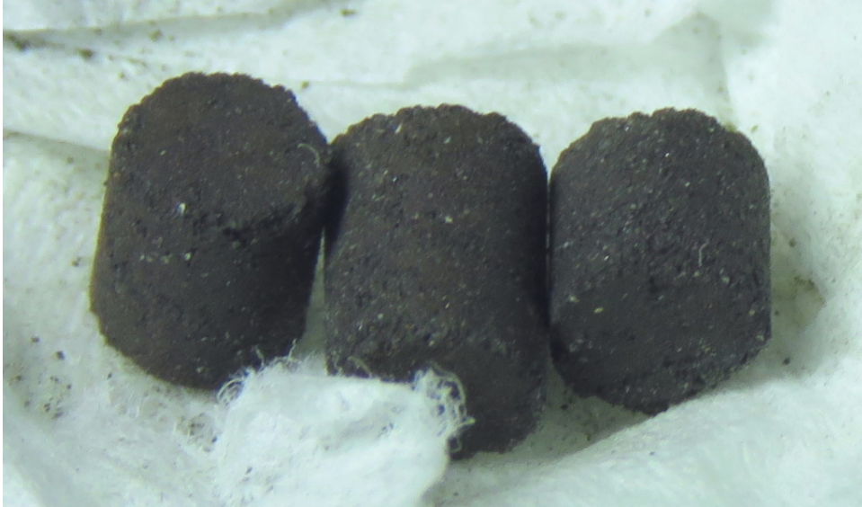
Final Pellets after run to 1100C in Vacuum.
