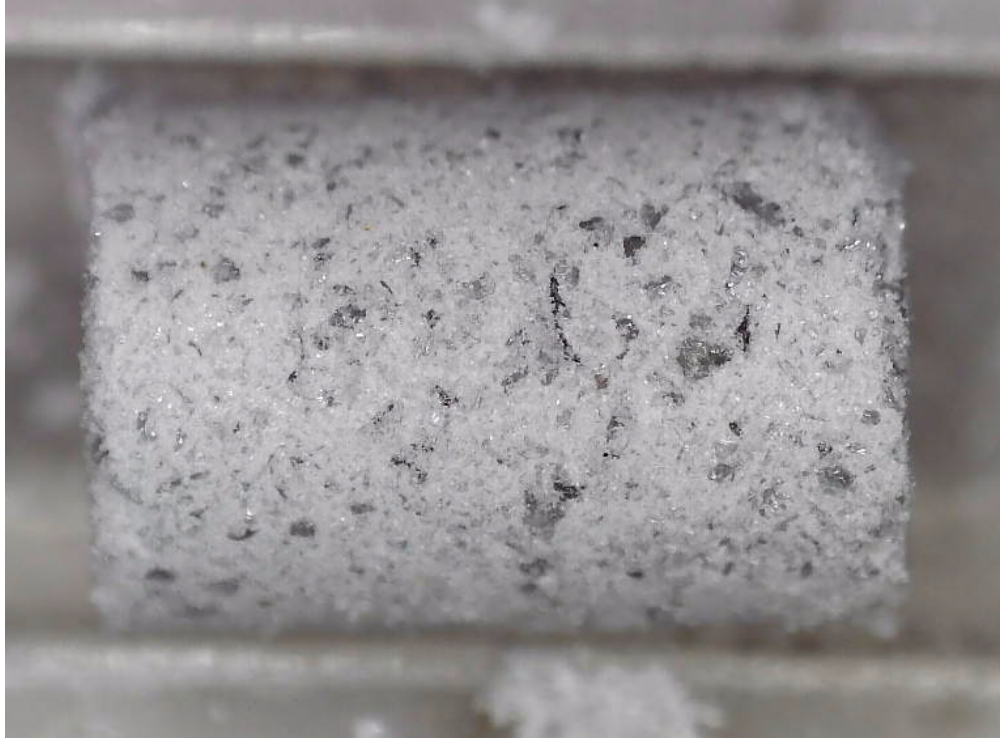
Initial 5M Glass ( Washington Mills) pellet - Pressed at ~ 30,000 psi
