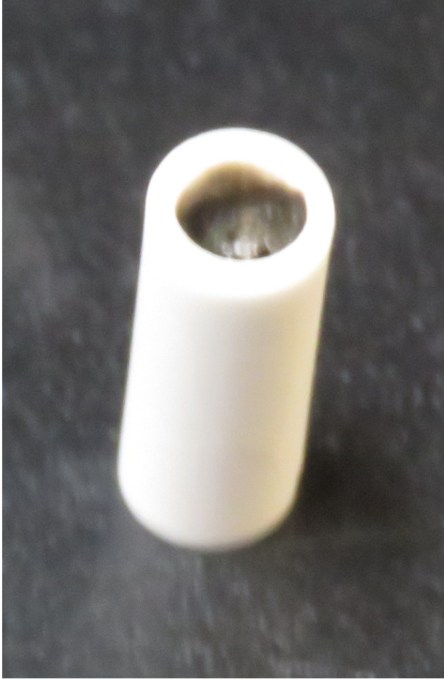
Crucible with test sample after run
