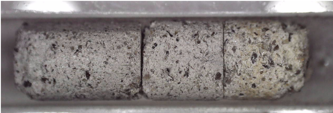
Final pellets after 2 nd run to 1000C in UHP argon on 5M Glass pellets from Matt Creedon
