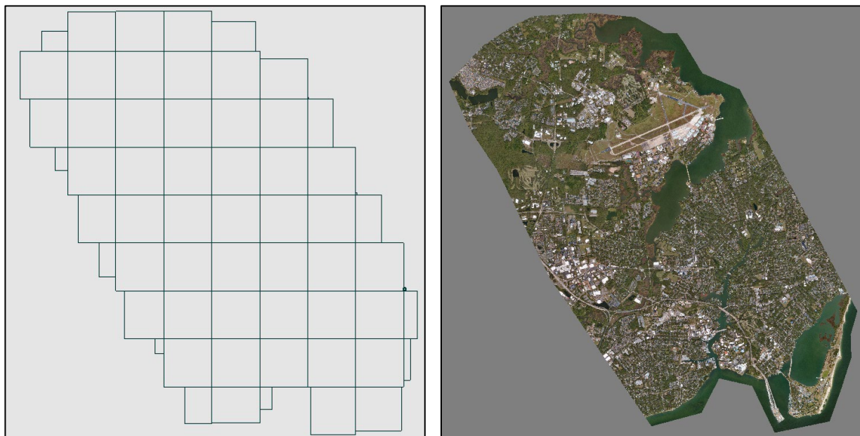
Fig. 3.3.2. Left: The 100 km 2 point cloud map area was partitioned into spatial tiles of size 2.25 km 2 or less. Right: Point clouds were colorized with spatially registered top-down imagery. Image sources: © 2023 Maxar Technologies.
