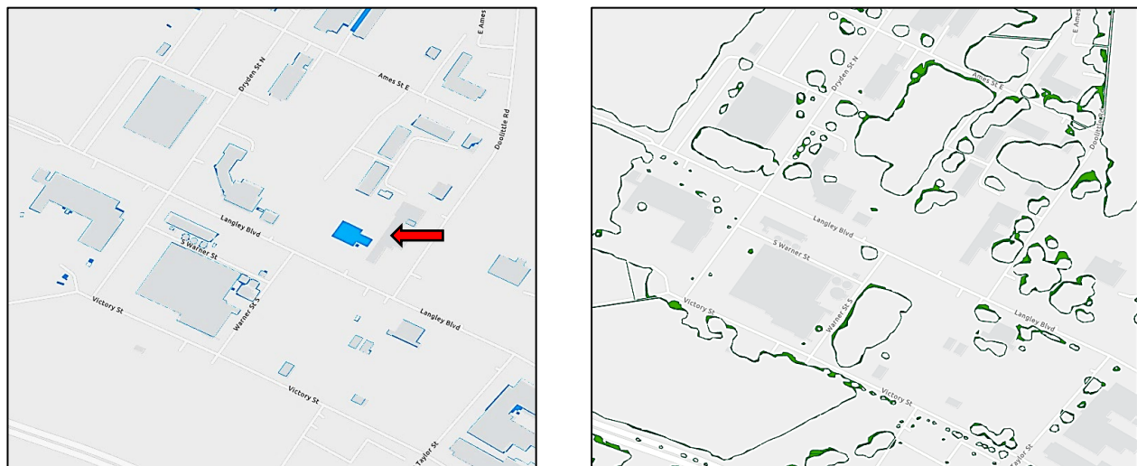
Fig 4.2.1.1 Top-down view of pairwise XOR of building layers (blue, left) and tree layers (green, right) to reveal differences across the time between the first two geodata deliveries. The XOR results are overlaid on a basemap with street names. Only thin (less than one meter) differences are seen for most buildings, which demonstrates meter-level placement consistency. Construction started on a new wind tunnel (the NASA Flight Dynamics Research Facility) in the time between map deliveries; this new structure is the solid blue shape at center left (red arrow). Tree and shrubby growth in the spring and summer are revealed in the foliage XOR at right. The horizontal length of both images is approximately 650 m. Image feature sources: NASA from features ©2023 Maxar Technologies. Base map sources: Base map sources: VGIN, Esri, TomTom, Garmin, SafeGraph, GeoTechnologies, Inc, METI/NASA, USGS, EPA, NPS, US Census Bureau, USDA, USFWS.
