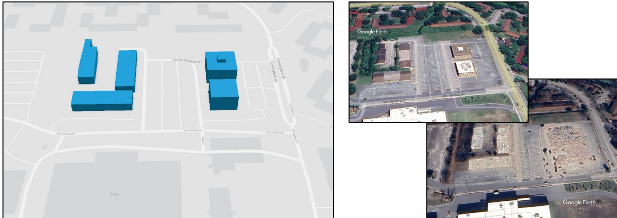
Fig. 4.2.4.2 Left: Building difference map for the time window from March 2024 to September 2024 shows a change on Von Schilling Drive in Hampton Virginia (76.3841494°W 37.0460990°N). Right: Google Earth historical imagery shows that building demolition occurred between November 2023 (top) and February 2024 (bottom). Left image feature sources: NASA from features ©2024 Maxar Technologies. Left image base map sources: VGIN, Esri, TomTom, Garmin, SafeGraph, GeoTechnologies, Inc, METI/NASA, USGS, EPA, NPS, US Census Bureau, USDA, USFWS. Right image sources: Google Earth, Image 2025 © Airbus.
