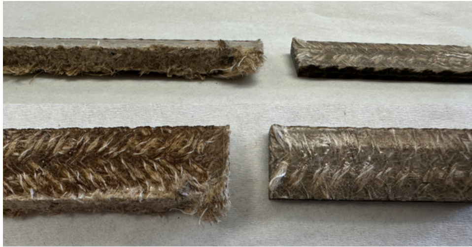
Figure 4.61 Braided flax/PLA samples after being cut on a wet diamond saw (left) and using a CO 2 laser (right).
