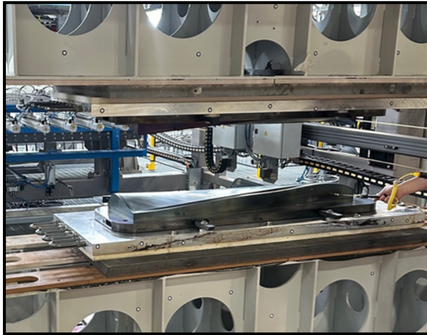
Figure 4.96 Hot press with propeller mold at NASA Ames Research Center High-Rate Manufacturing facility.
