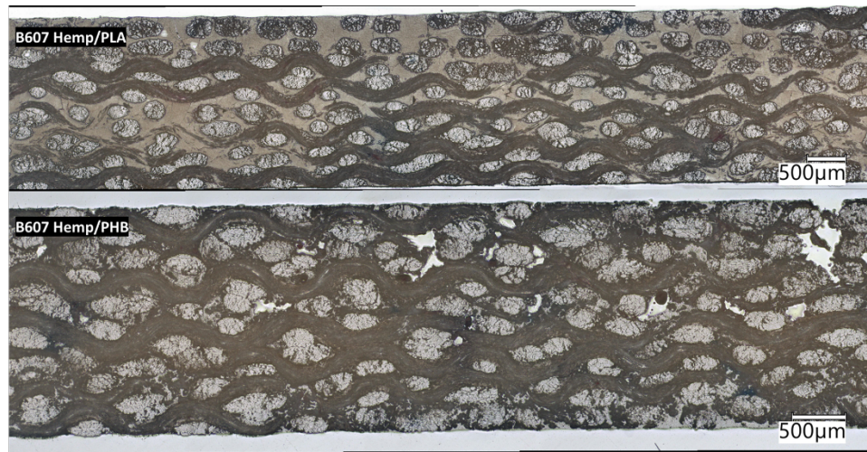
Figure 4.53 Optical microscope images at 100X of hemp/PLA cross section (top) and hemp/PHB (bottom) cross sections. Both iterations had some voids and regions of resin pooling, but generally were well consolidated.
