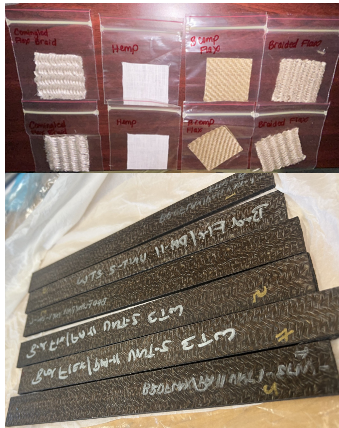
Figure 4.8 Moisture uptake samples: (top) natural fiber fabrics – flax-PA11 commingled fabric, hemp fabric, Bcomp woven flax fabric, braided flax fabric; (bottom) braided flax-PA11 composite coupons.
