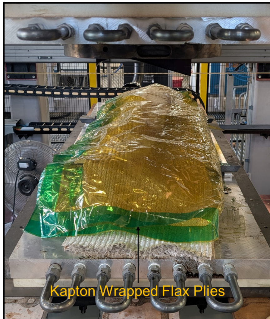
Figure 4.97 Propeller mold with Kapton wrapped commingled flax braid PA11 plies prepared for pressing.
