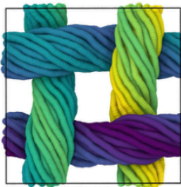
Figure 4.150. Four examples of (bottom) relaxed simulations that match the pattern (including plain, twill and triaxial braid), yarn ply (1 to 2), and yarn twist from visual inspection of (top) optical microscopy.
