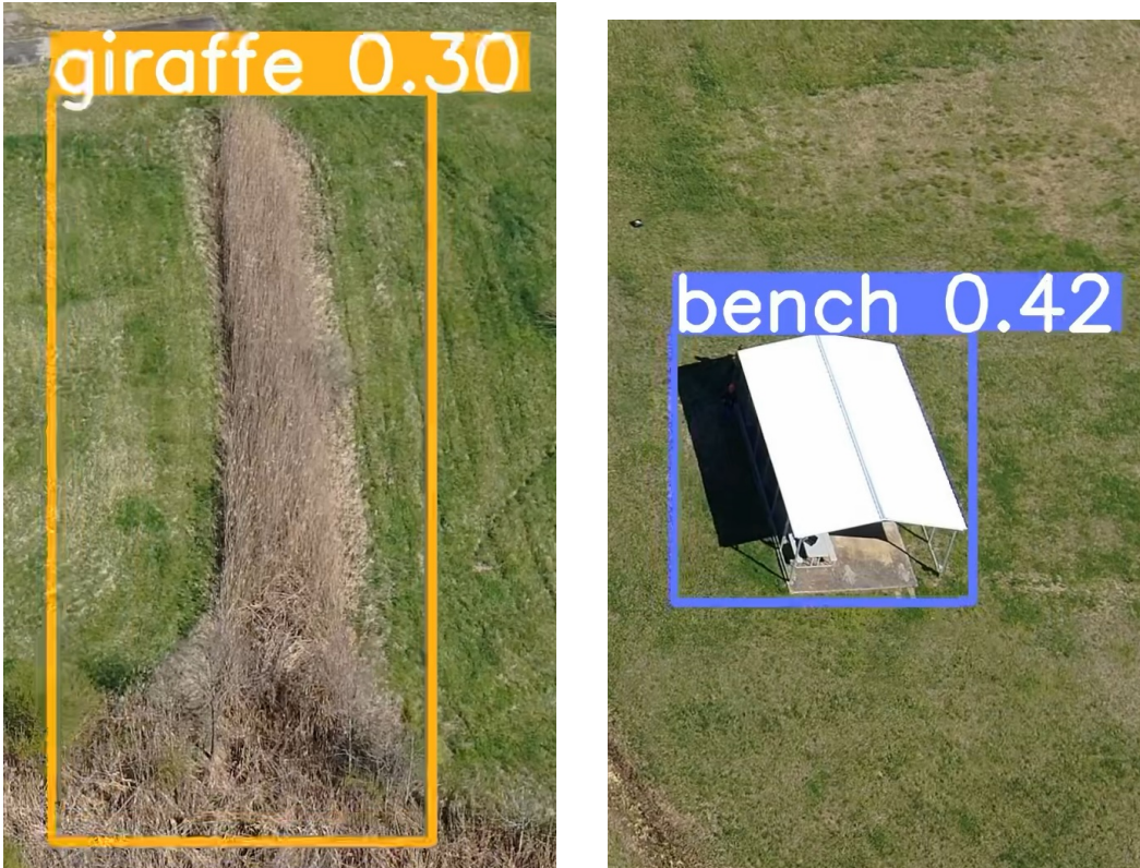
Figure 21: OOTB classifier (YOLOv8) trained on non-aerial data attempting to process aerial data
