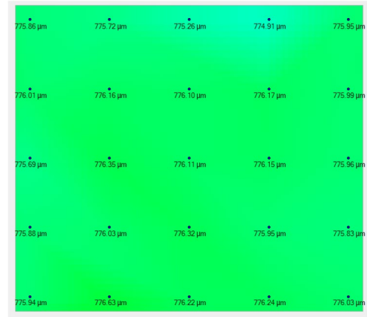
Figure 3: Pre-thinned TI TDA4VM die depth map measured by Sage Analytical
