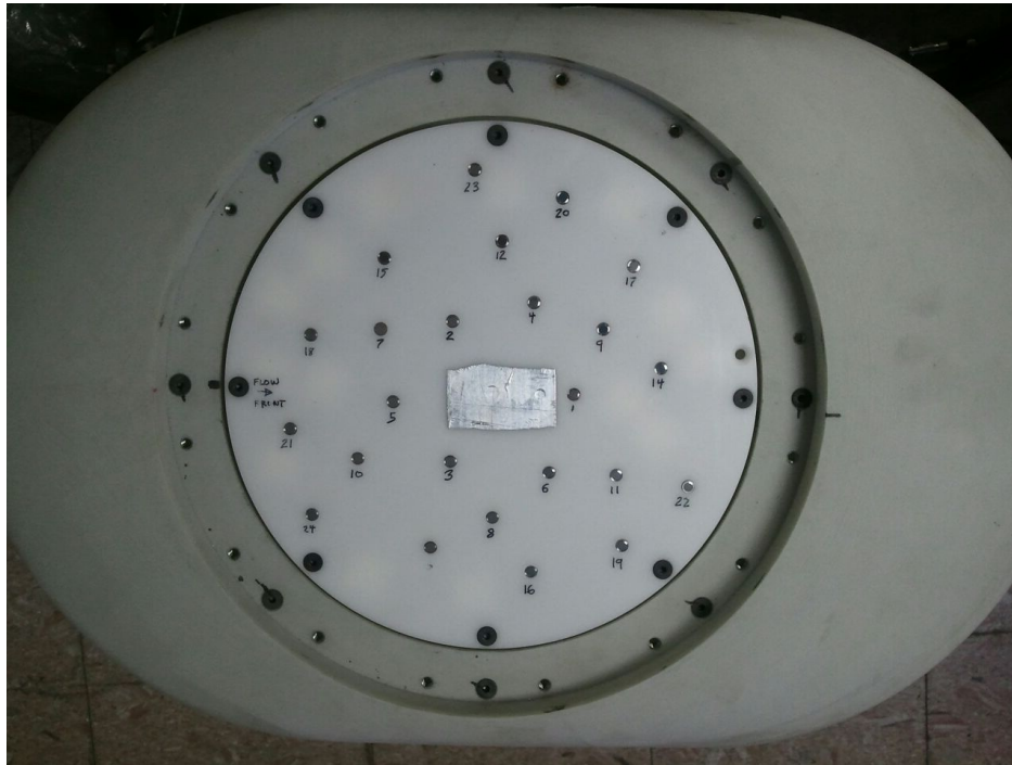
Figure 31. —Front view of 8-inch array with microphones flush mounted in a non-conductive plate.
