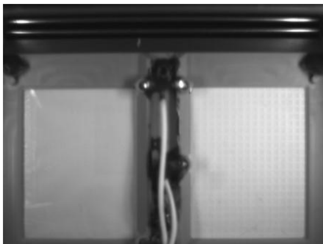
Figure 1. A glass in-plane interdigitated-electrode EDS (left), a thermal-radiator out-of-plane grid-electrode EDS (right), and one set of reduster EDS bars (top). This image was taken with the payload camera as the lander travelled to the moon.
