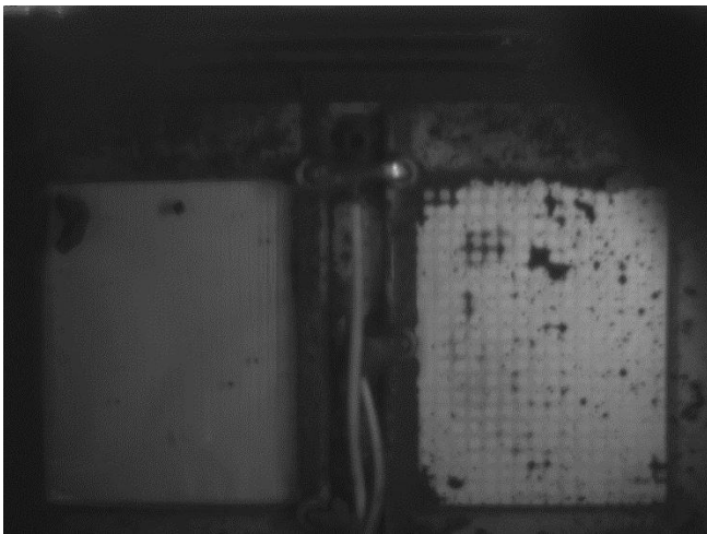
Figure 4. The EDSs shown in Figure 3, after operation to remove the dust. The glass EDS (left) removed 97% of the dust while the thermal-radiator EDS removed 82%.
