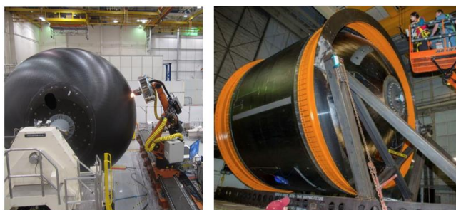
Figure 8 CCTD 5.5m Tanking in Fabrication (Left) and being shipped for testing (Right) [3]
