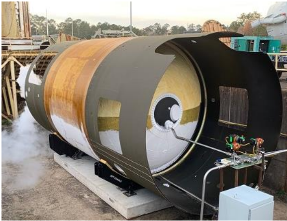
Figure 9 XSP Composite Tank During Testing [4]
