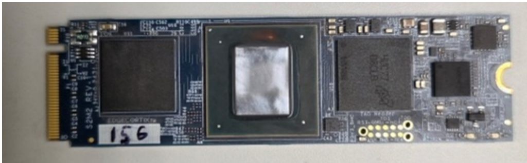
Figure 2: De-lidded and thinned SAKURA-II card
