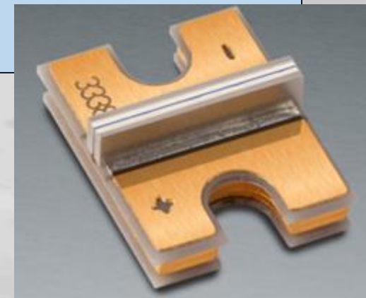
Example of high-efficiency semiconductor bar laser
