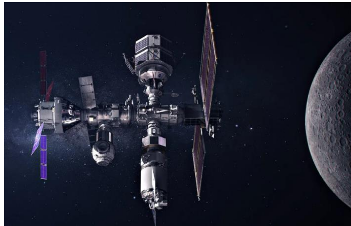
Gateway: The spaceship in lunar orbit where astronauts will transfer between Orion and the lander on regular Artemis missions. Gateway will remain in orbit for more than a decade, providing a place to live and work, and supporting long-term science and human exploration on and around the Moon.
