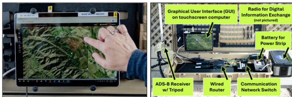
Figure 1. Building a volume on the GUI (left) and the field-deployable PAMS Case (right).
