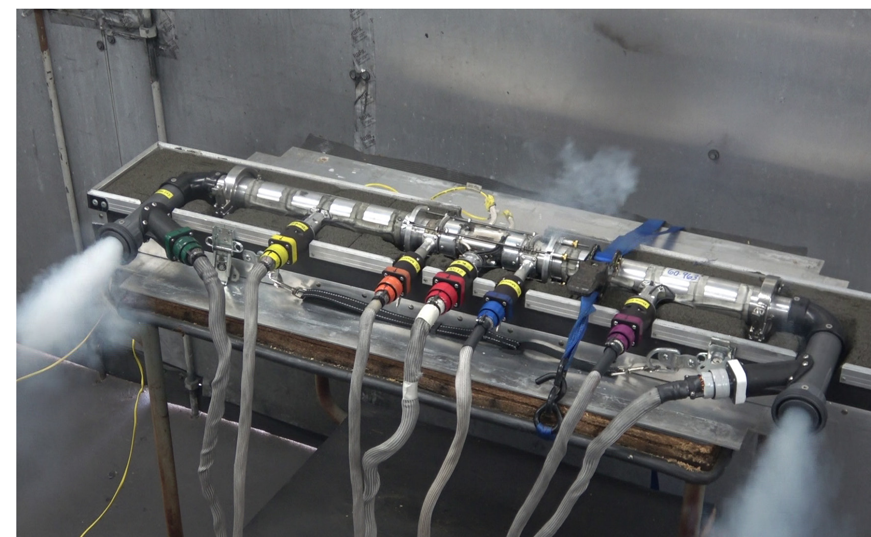
The S-FTRC during a battery test with a cell going into thermal runaway with gases ejected from the exhaust.
