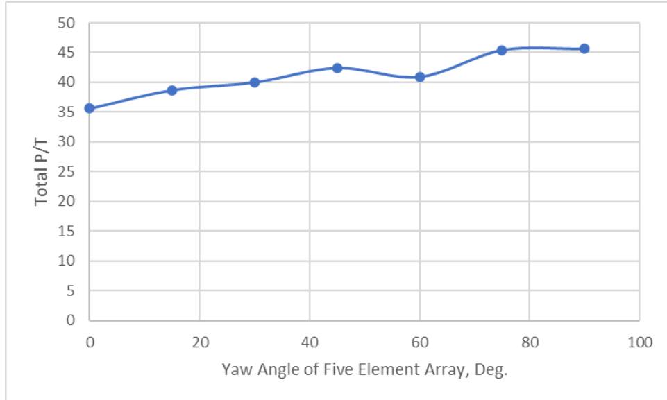
Figure 32. Average P/T ratio as a function of yaw angle for five rotor element array for advance ratio of 0.033 (constant collective for all rotors of 10Deg. and zero pitch angle)
