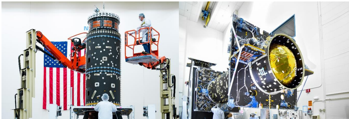
Figure 6. PPE electric propulsion build showing an 825L Xenon tank being installed [16] (left), and after the tanks have been installed [17] (right).
