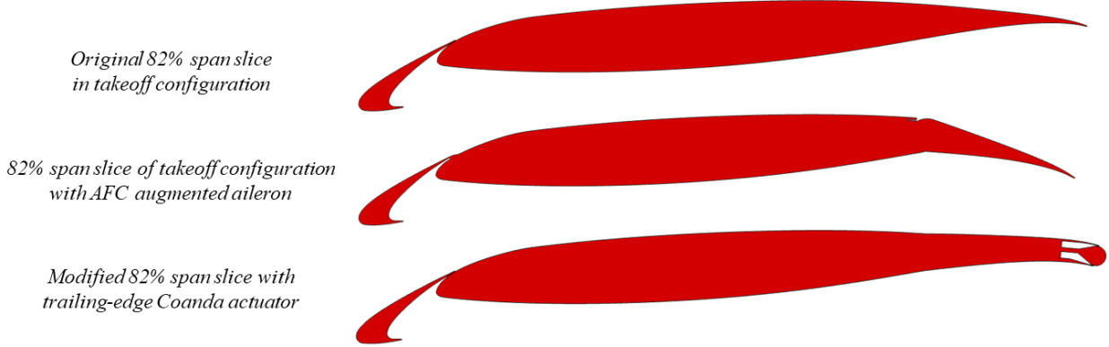
Fig. 2 Two-dimensional cross-sections of the CRM-HL at 82% span for (top) original geometry, (middle) AFC-augmented aileron, and (bottom) installed trailing-edge Coanda actuator
