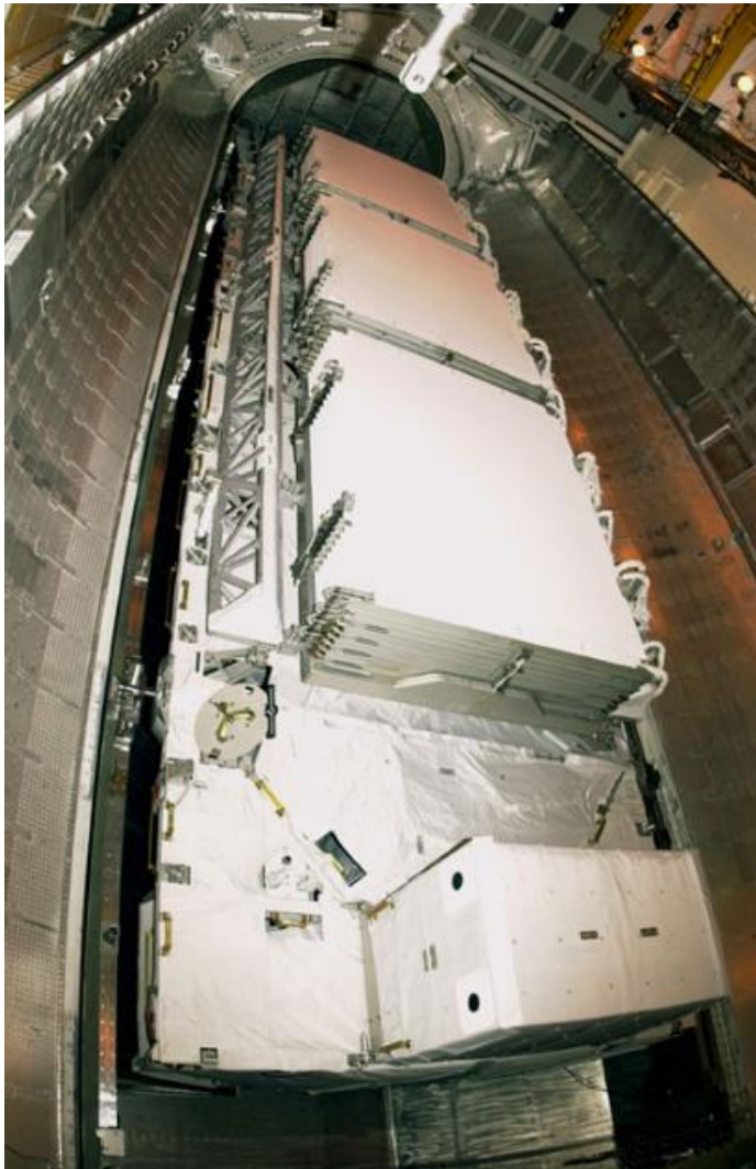
Radiator Unit Stowed in the Space Shuttle for delivery
