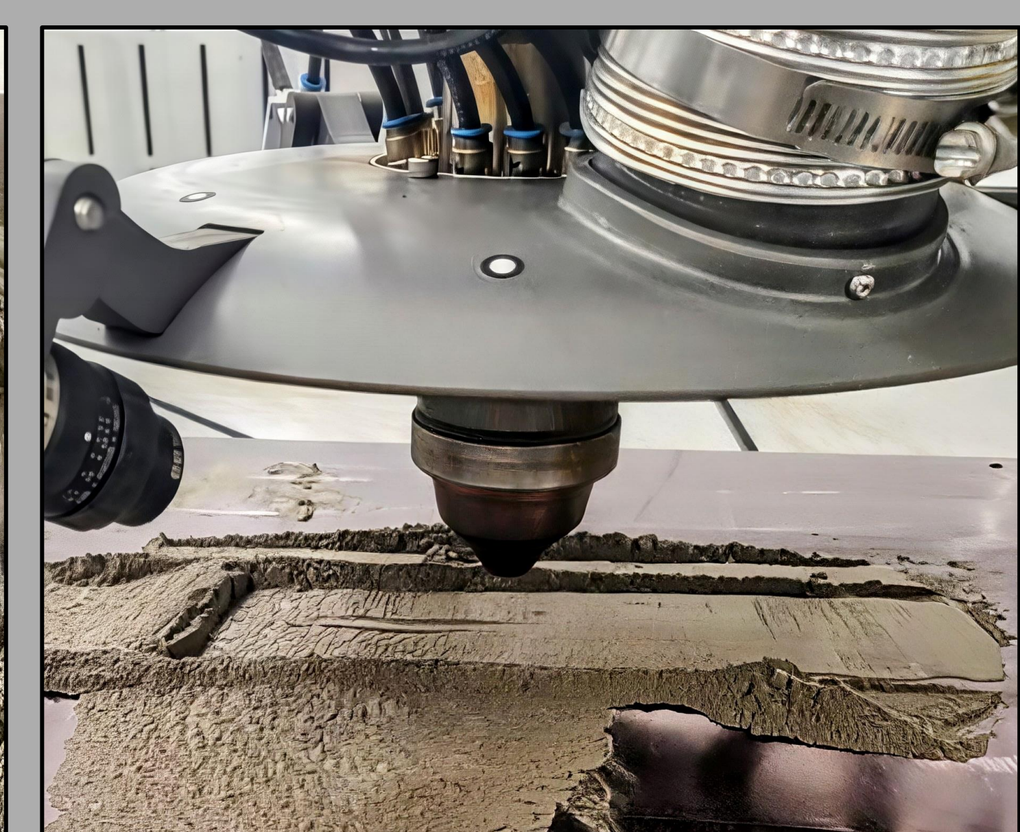
Laser Consolidated Lunar Regolith Simulant using Directed Energy Deposition
