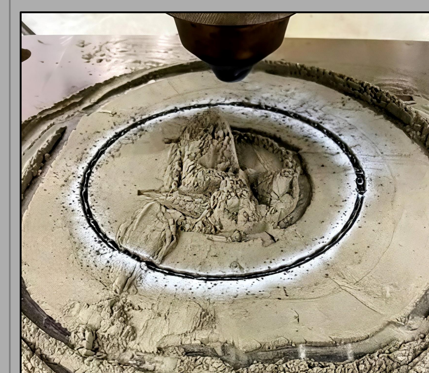
Laser Consolidated Lunar Regolith Simulant using Directed Energy Deposition
