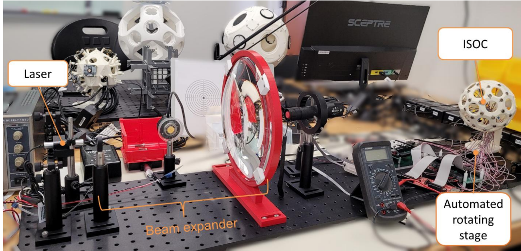
Figure 6. Picture of an early AoA measuring system setup where one can observe the laser illuminator (beam expander), an ISOC and an automated rotating stage.
