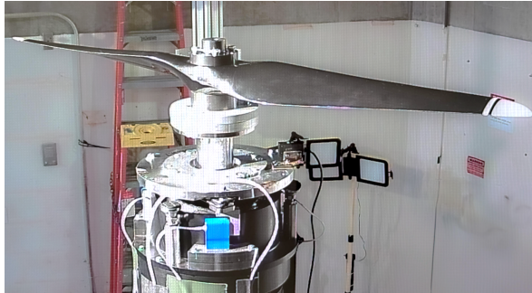
(a) Thrust check setup with AWT propeller installed on shaft of ROAMX stand.
