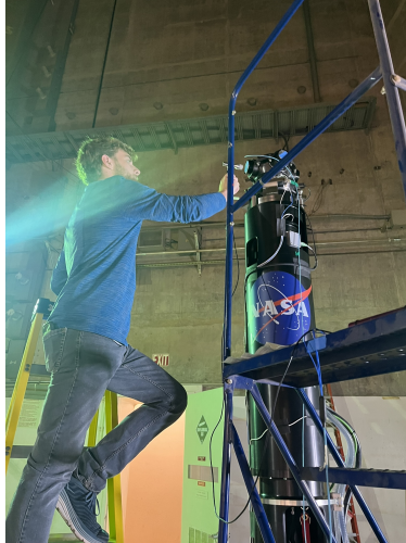
Fig. 22 Ground vibration test for ROAMX test stand in PAL.
