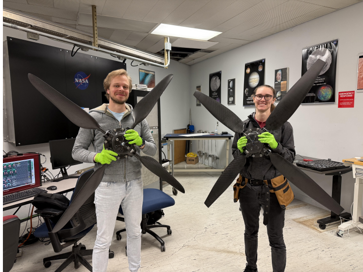
Fig. 16 Ingenuity and ROAMX blades installed on DUC hub.
