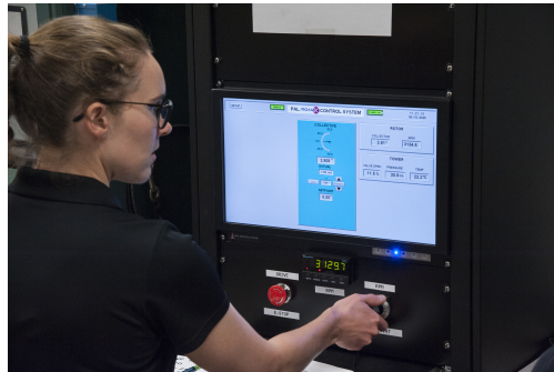
Fig. 20 Control console, potentiometer, and RPM display for rotor.
