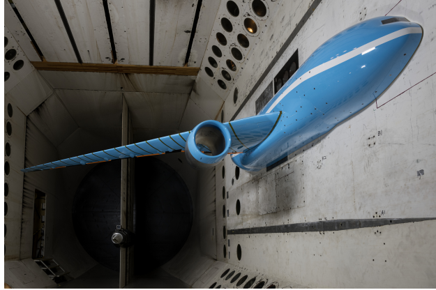
Fig. 1 The IAWTM wind tunnel model (credit: NASA / Mark Knopp).
