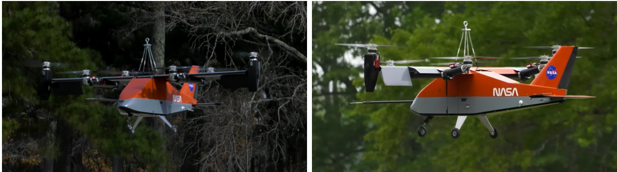
Fig. 10 RAVEN-SWFT hover free-flight testing. (Credit: NASA)
