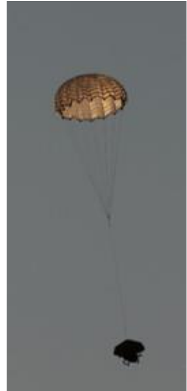
Fig. 3 Drone Drop Tests of the Posed configuration with the main parachute deployed.
