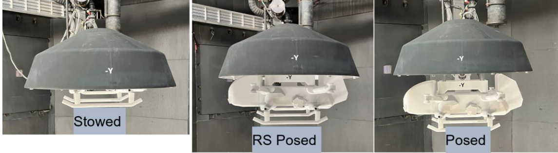
Fig. 18 Sideview of the 15.56%-scale models of the Stowed, RS Posed, and Posed configurations mounted for pitch oscillations in the VST to show the relative position of the Lander to the backshell.
