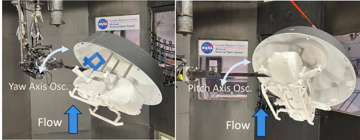
Fig. 9 15.56%-scale model of the Posed configuration mounted for pitch and yaw axis forced oscillation testing.
