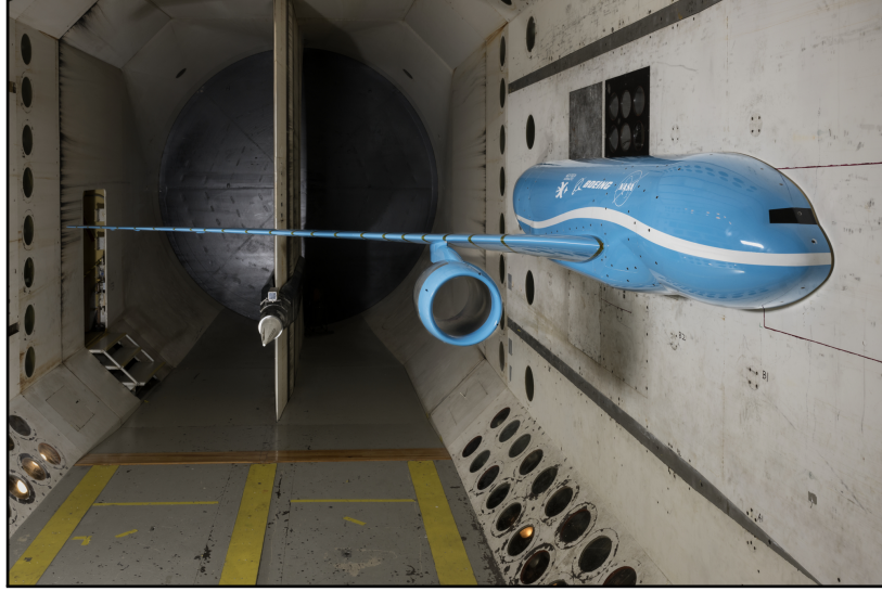
Fig. 1 IAWTM wind-tunnel model installed in the Transonic Dynamics Tunnel during Entry 1 [Source: NASA].
