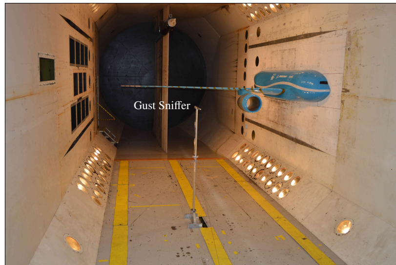
Fig. 7 Gust sniffer probe located upstream of the IAWTM wind-tunnel model during Entry 2 [Source: NASA].
