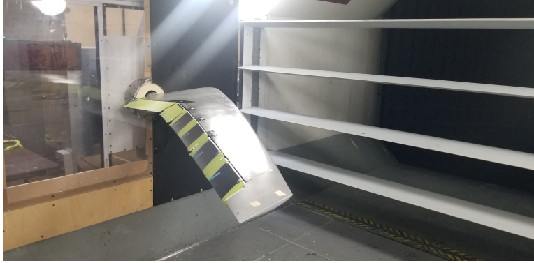
Fig. 1 Large Flexible Wing In Kirsten Wind Tunnel Test Section
