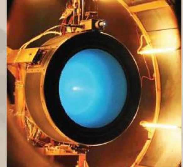
NEXT-C Thermal-Vacuum Testing
