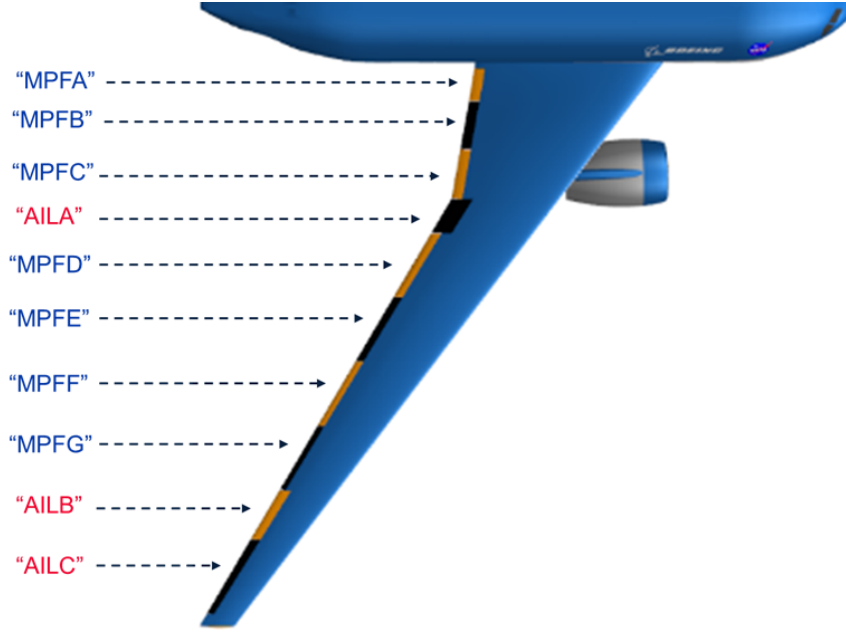
Fig. 5 Wind-tunnel model control surfaces and major components.
