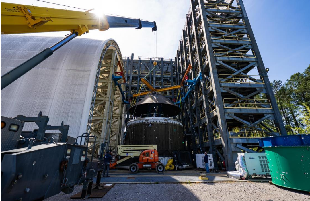
Figure 7: The Block 1B and Block 2 payload adapter underwent structural evaluation testing at NASA Marshall. The engineering development unit was then moved into storage.
