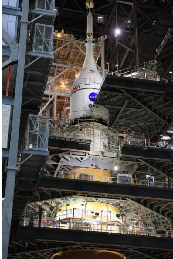
Figure 1: The Artemis II SLS and Orion are stacked in NASA's Vehicle Assembly Building at NASA's Kennedy Space Center.
