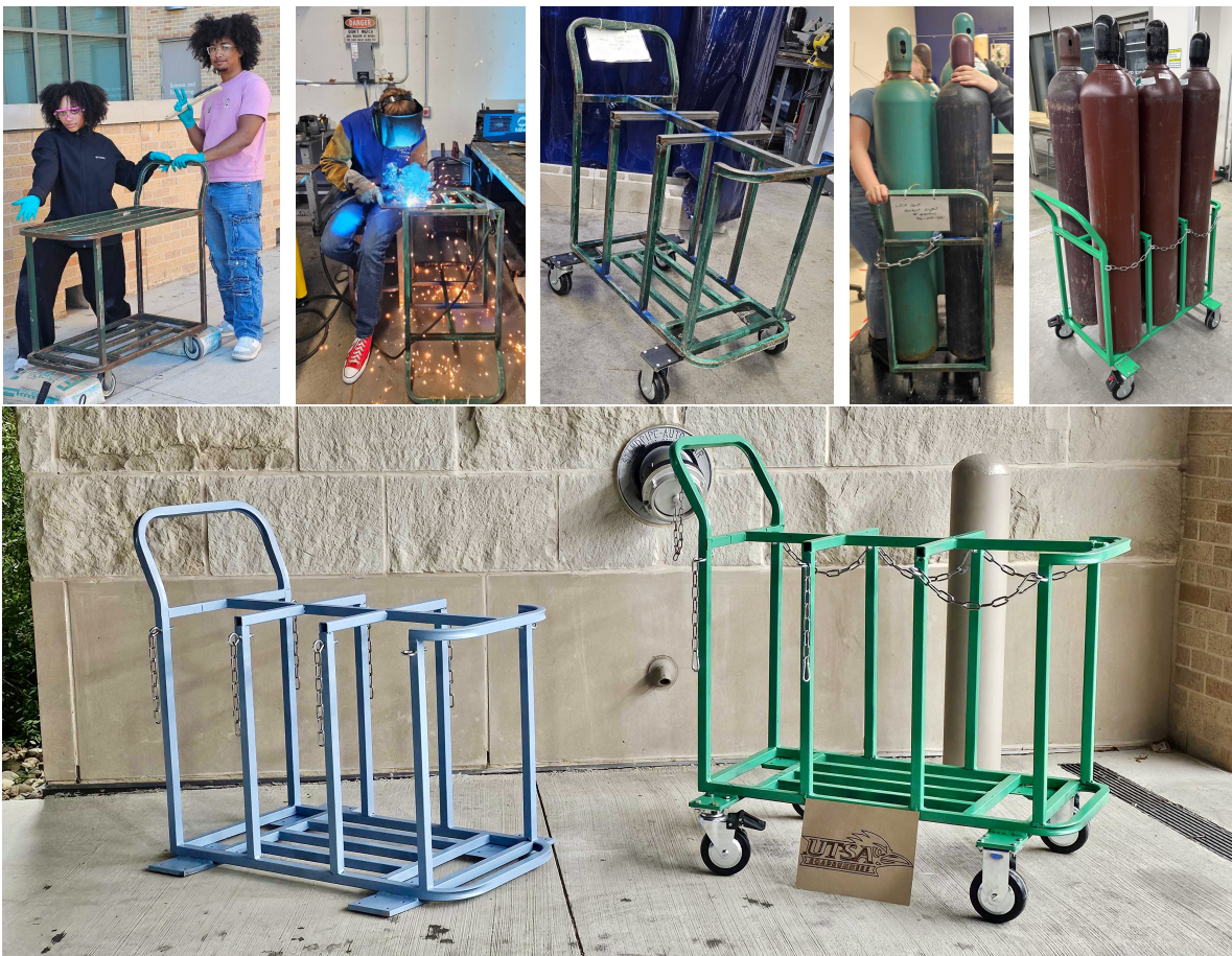
Fig. 27 Conversion of bread carts to propellant K-bottle 6-packs
