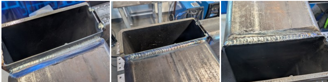
Fig. 9 Root pass (left), Fill pass (middle), Cap pass (right)
