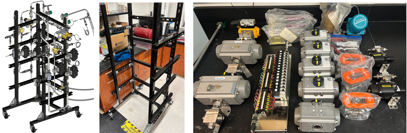
Fig. 25 Fluid system CAD render ( left ), stand structure ( middle ), and valve hardware ( right ).
