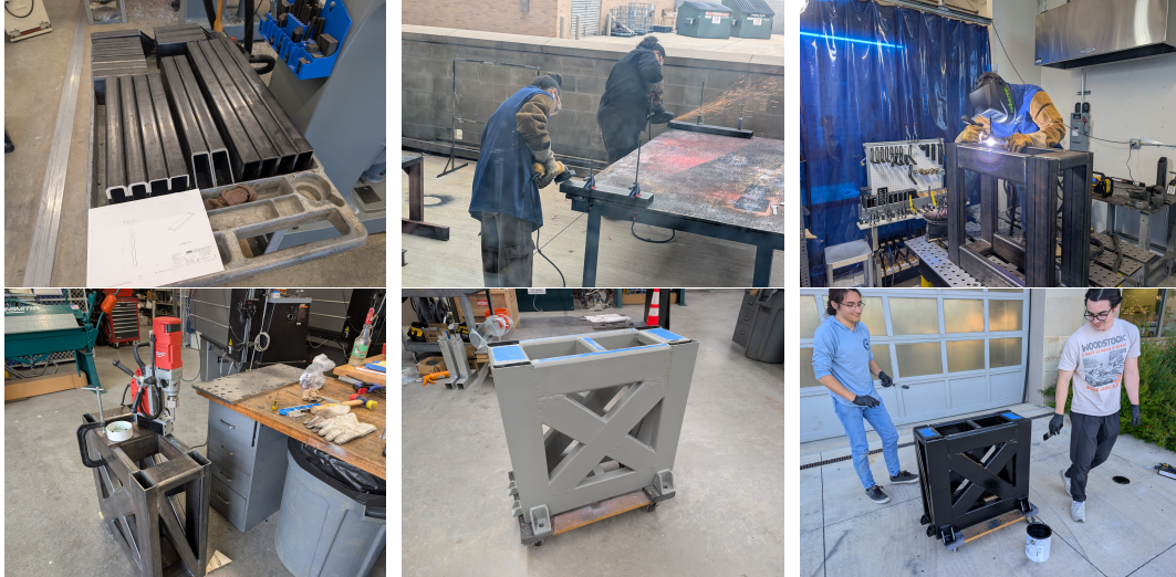
Fig. 22 Photographs of the base structure fabrication process.
