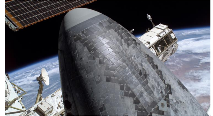
Space Shuttle Discovery TPS Tiles
