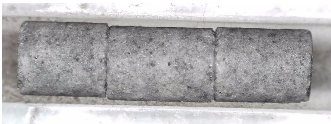
The final, joined, pellets ( after the run to 1400 C in 4% hydrogen/argon).
