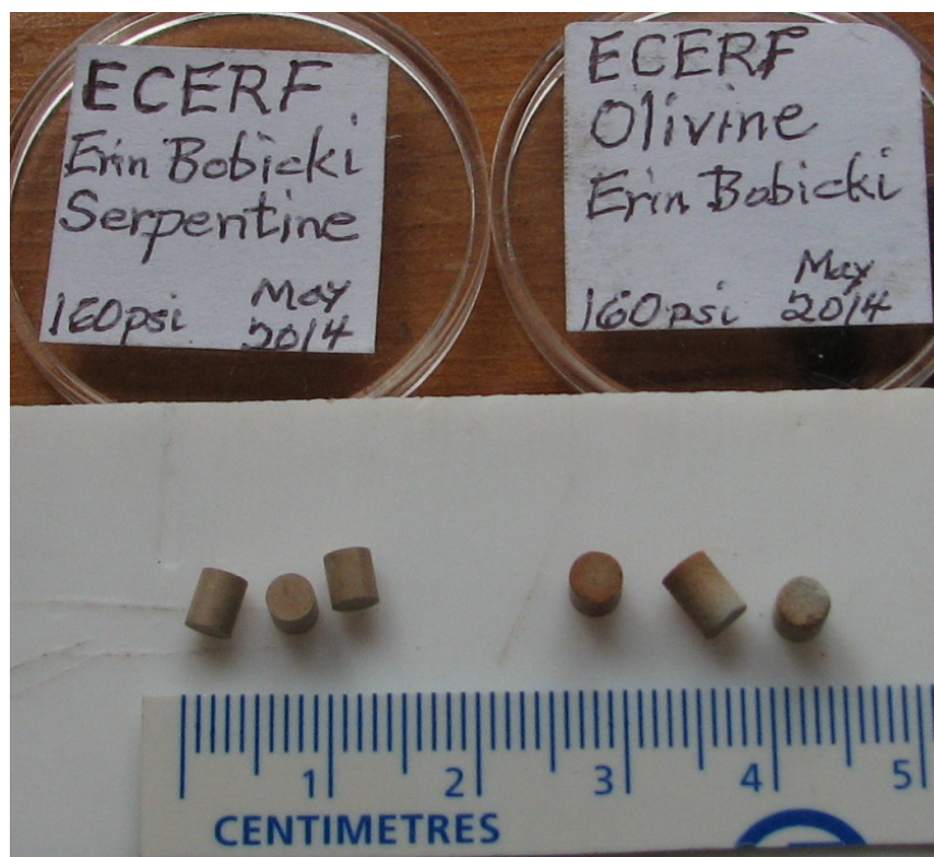
Final serpentine and olivine pellets.
