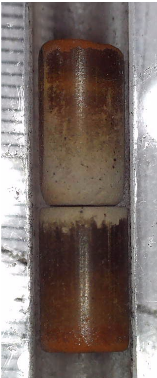
One initial pellet in flowing UHP nitrogen.
