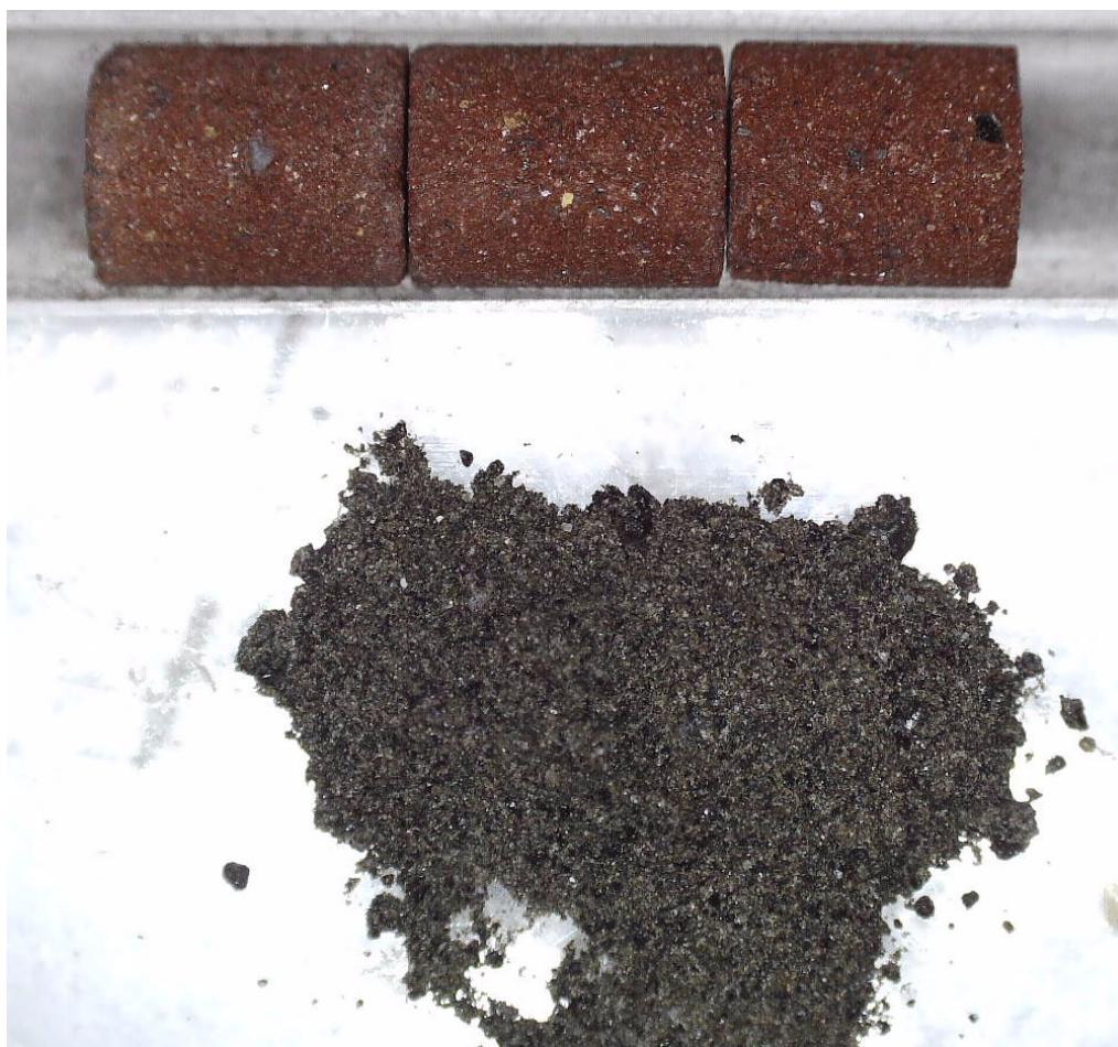
Comparison of the colour of the initial powder with that of the final pellets after the run to 1100 C in 4% hydrogen/Argon.
