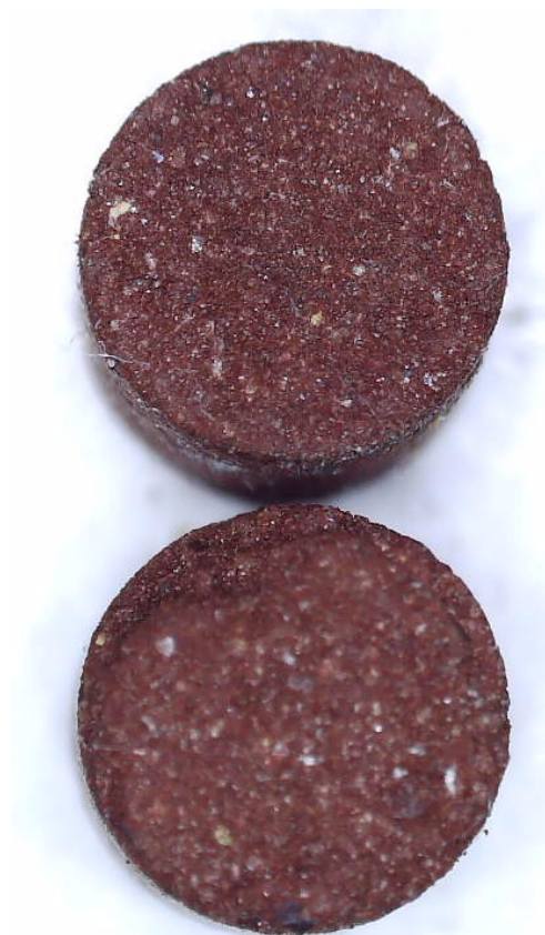
Cut faces of the “cut” final pellet
