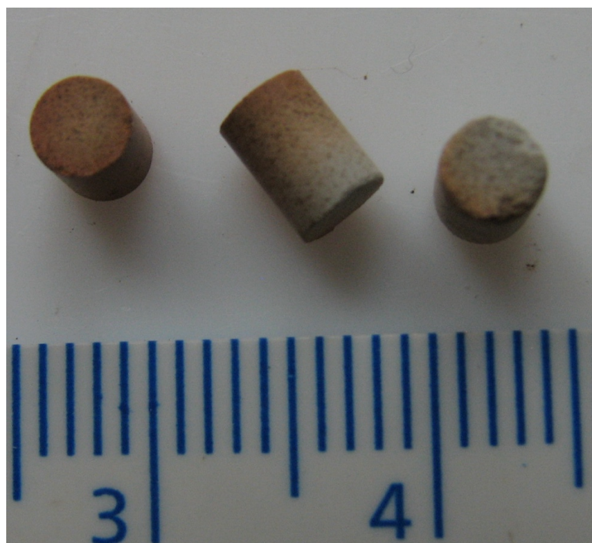
Final Olivine pellets. Bottom pellet had brown/orange exterior. Mid pellet partially brow.
