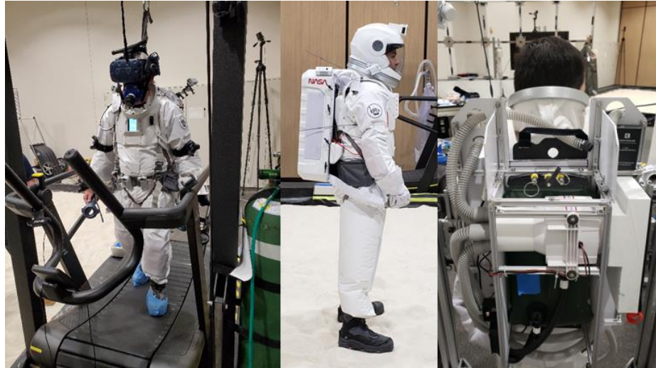
Figure 2-7. HS3 operating in APACHE space
