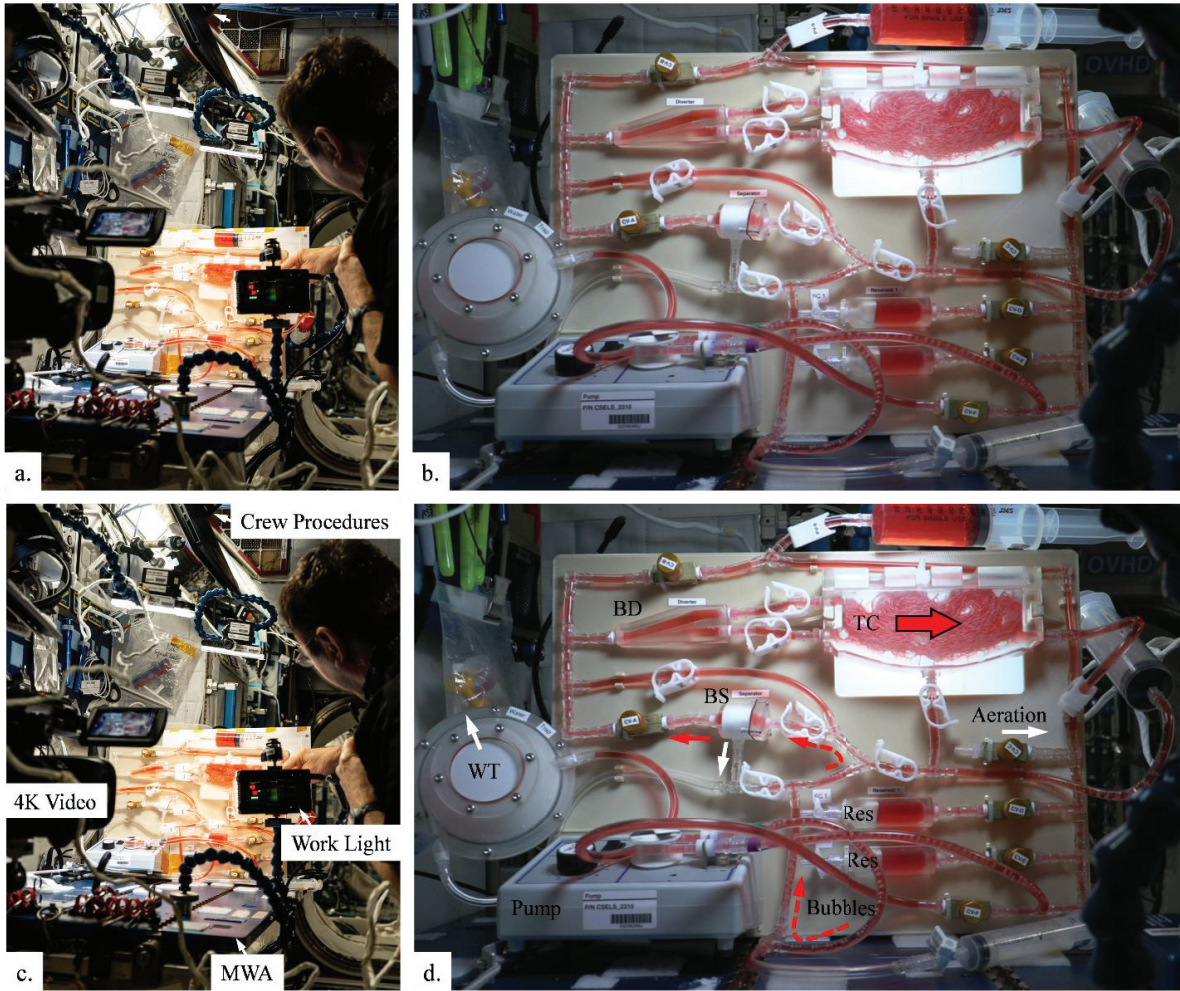
Figure 1. a. Typical over-the-shoulder camera image of Astronaut Michael Barrett conducting PWM-5b on the MWA. b. Image of PWM-5b from primary 4K video cameras during demonstrations of steady Hydroponic Flow with Aeration, Bubble Separation, Water Trap, and Bubble Diversion through the wedge Test Channel (TC) with packed Root R4. Respective labels provided in c. and d. Plant root models R1-R4 are readily removed and replaced.
