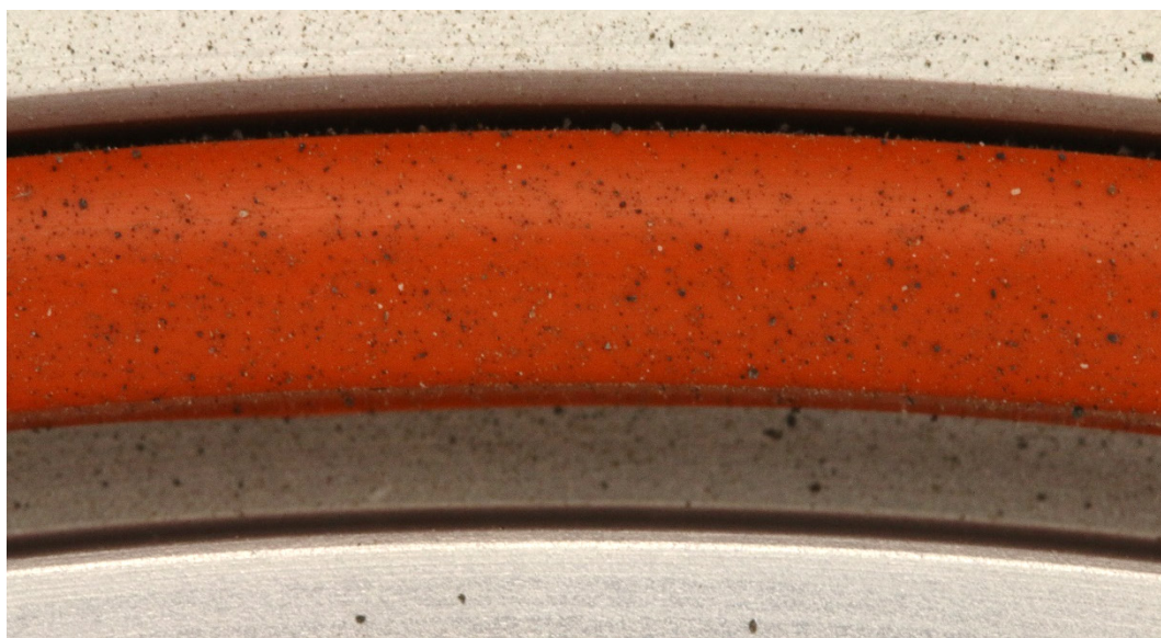
Figure 1.—Macroscopic image of dust on a NASA Docking System (NDS) seal post-deposition.
