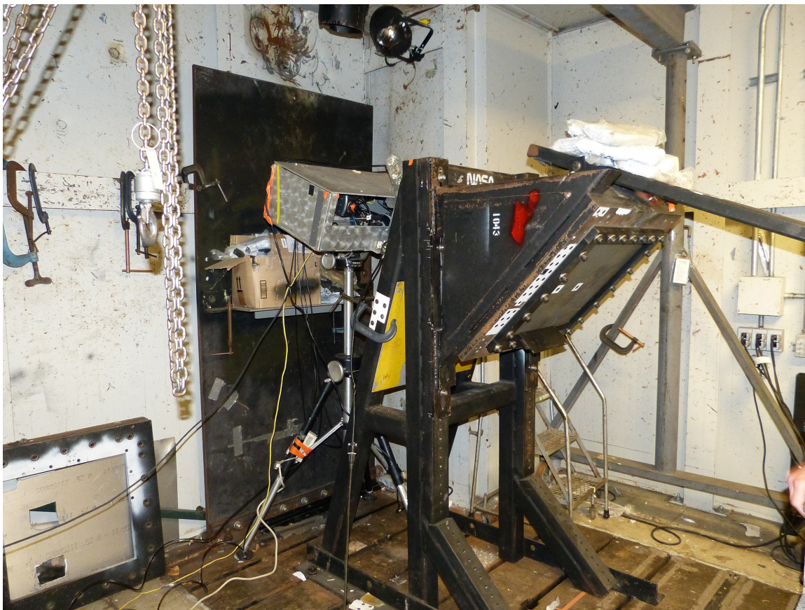
Figure 9.—Large panel test setup showing orientation of projectile and test specimen.
