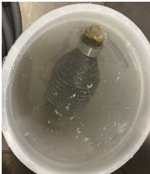
Figure 18.—Mandrel being washed out in water bucket; entire CF shaft assembly was left to soak in bucket for 1 h until fully washed out.
