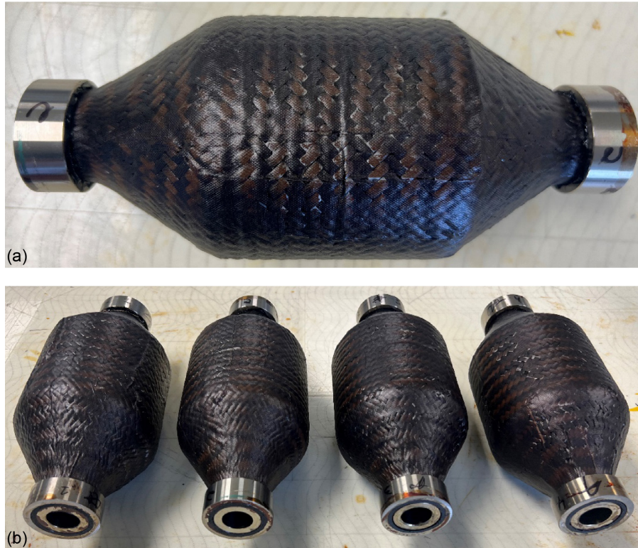
Figure 20.—Completed carbon fiber mandrels, all using hybrid fabric overwrap method; bearings installed on ends. (a) One finished part laid horizontally. (b) All four parts next to each other. Shafts had average mass of 140 g without bearings. Combined weight of four bearings was 248 g. Total system mass (shaft plus bearing) was 387 g per finished part.
