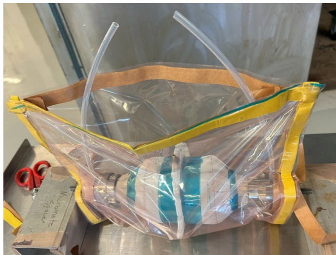
Figure 15.—Vacuum bagging with part enveloped; not yet sealed.
