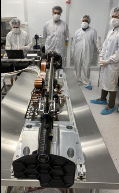
Subsurface excavation TRIDENT Drill
