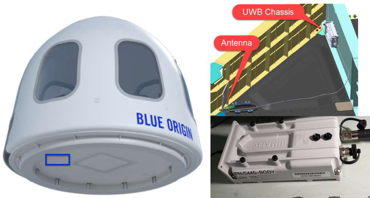
Figure 3: One UWB sensor installed in the aft portion of the New Shepard Crew Capsule. The UWB antenna was installed behind an aft-facing window near the edge of Crew Capsule base heat shield with the UWB sensor chassis installed on a nearby structural member.
