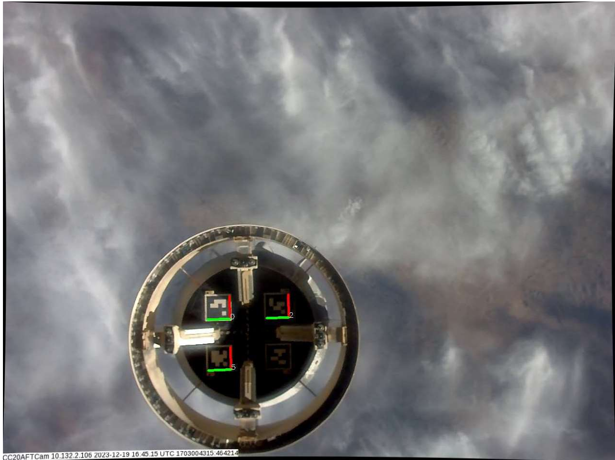
Figure 16: AprilTags detected in one frame of the CC aft camera.
