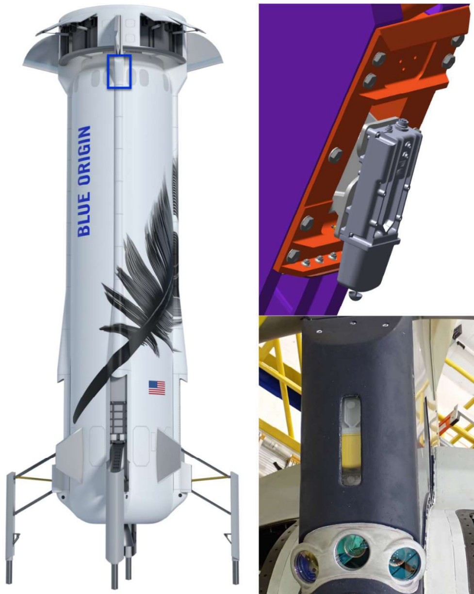
Figure 8: One UWB sensor was installed in a New Shepard Propulsion Module ring-fin support (marked by the blue box), providing a view of the ground.
