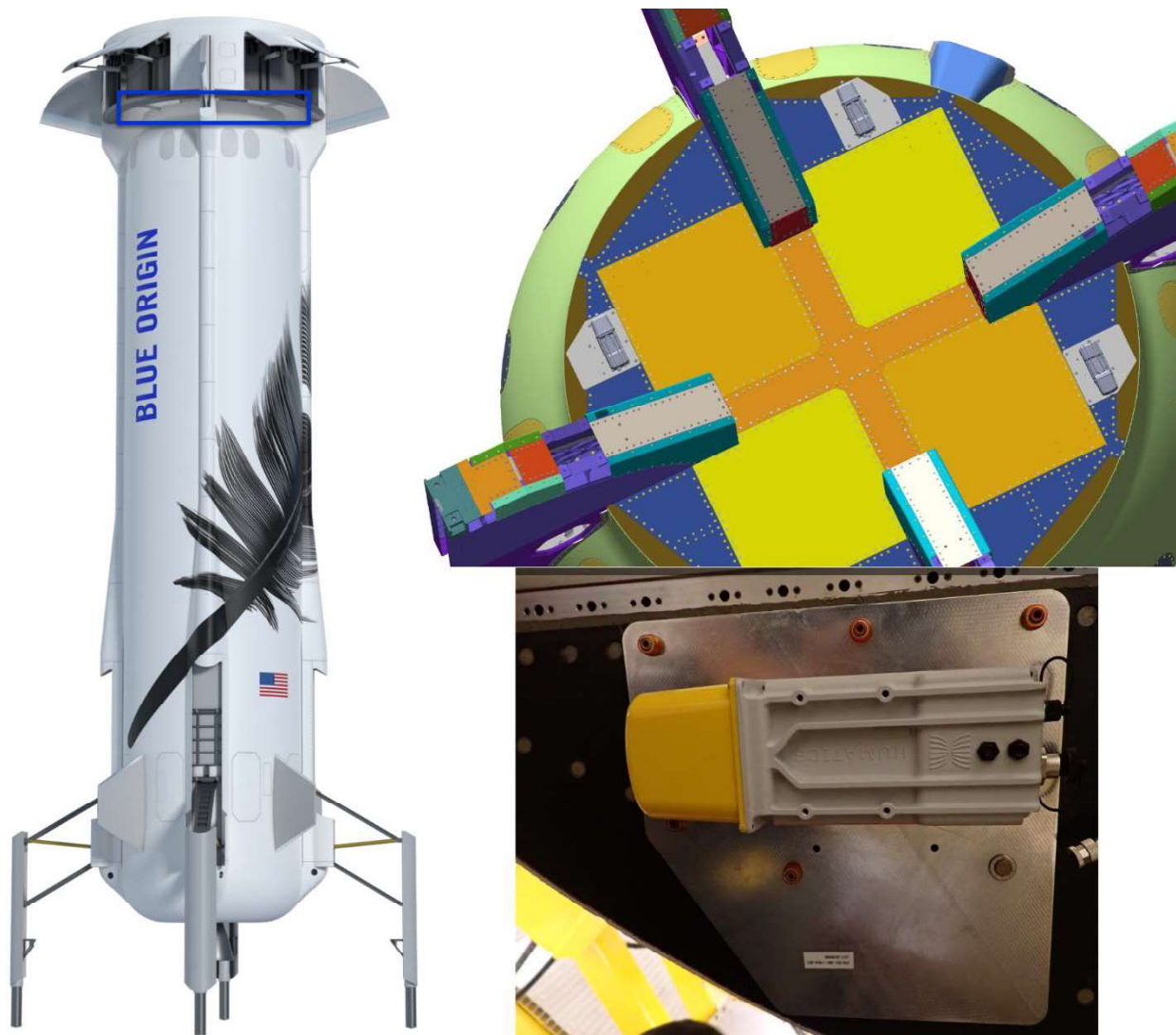
Figure 2: Three UWB sensors installed on the top of the New Shepard Propulsion Module (blue boxed area), distributed to provide as wide as possible of a ranging baseline.
