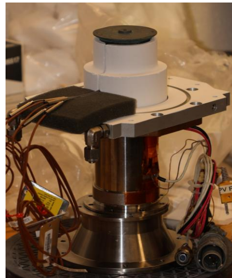
Figure 10. ASC convertor with thermocouples and insulation installed
