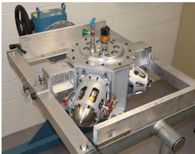
Figure 12. Assembled Pu-238 SG Testbed in the assembly fixture
