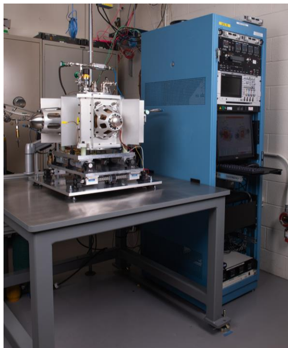
Figure 13. Pu-238 SG Testbed integrated on the test stand. For scale, blue test rack is standard height of 42 U (1.87 m)
