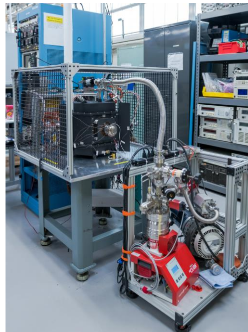
Figure 18. Fully assembled Am-241 SG Testbed mounted on to the test stand
