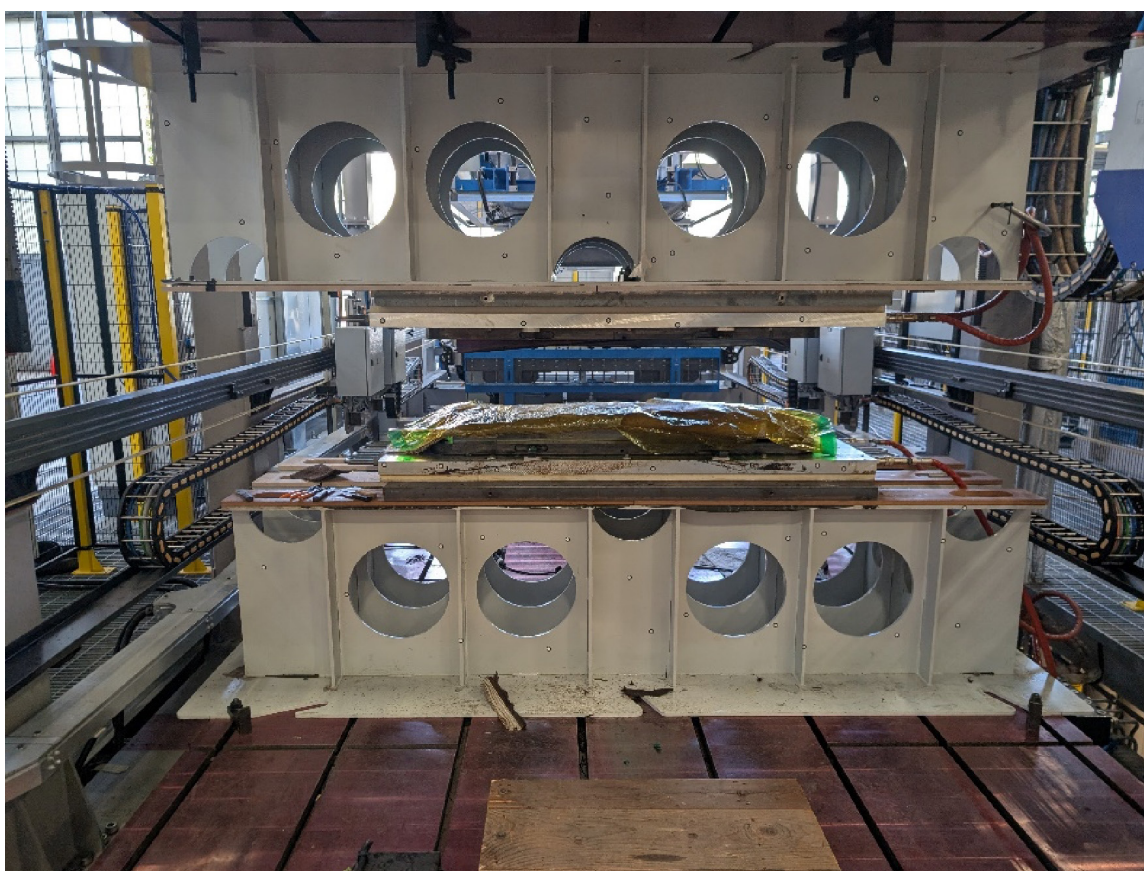
Figure 7.—Composite layup in between mold-release-coated polyimide release liner.
