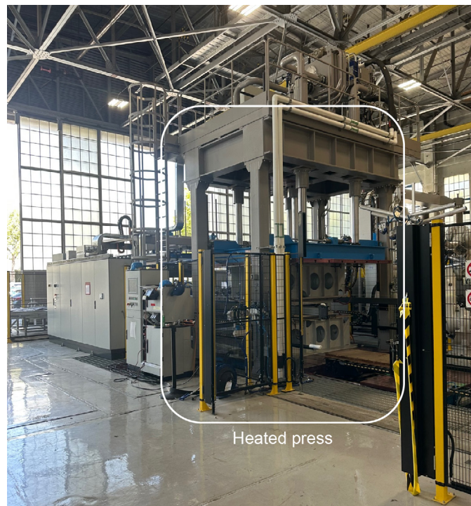
Figure 3.—Preformer line at the AHRCM with heated press used for propeller manufacturing.
