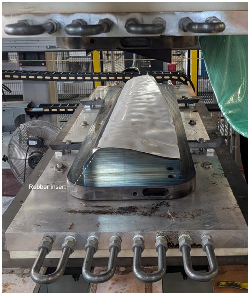
Figure 10.—Rubber insert gap filler used to evenly distribute pressure of mold.
