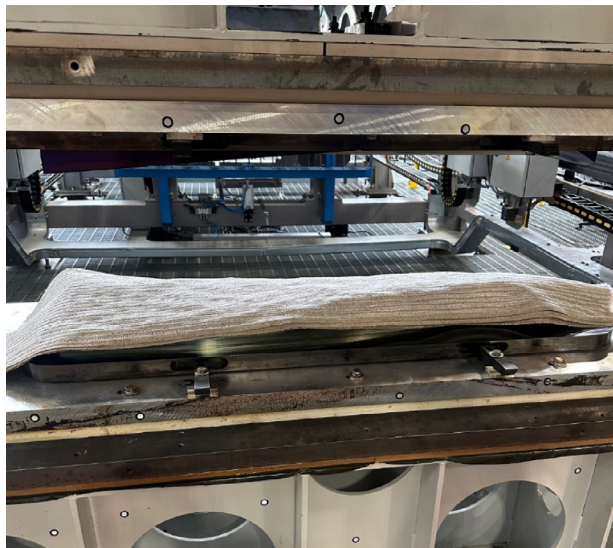
Figure 5.—Flax plies laid up directly on compression mold.
