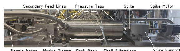
Figure 4 – The XE-2.2 prototype installed at Purdue University.
