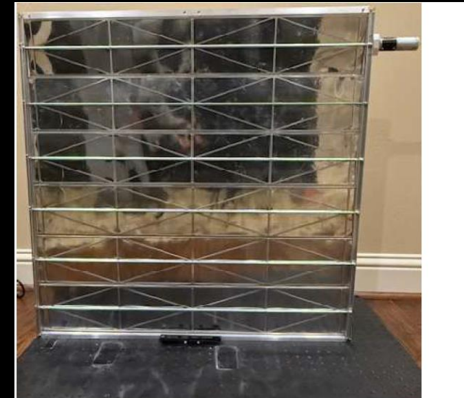
(b) View from the back of louver module with vanes in closed position.
