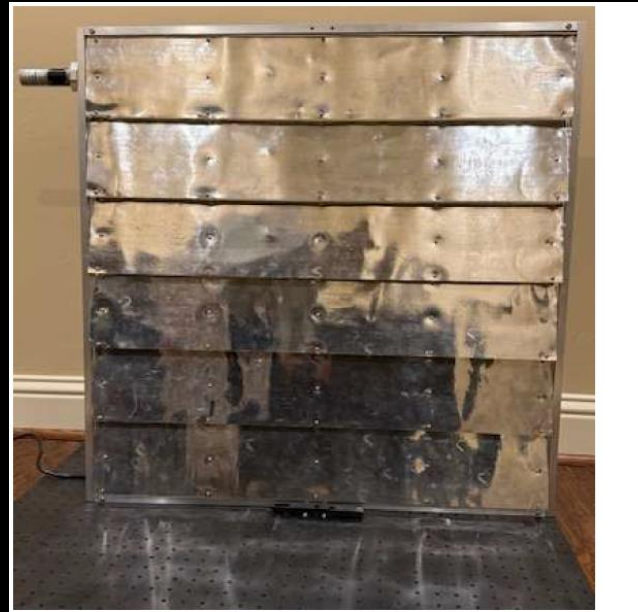
(a) View from the front of louver module with vanes in closed position.
