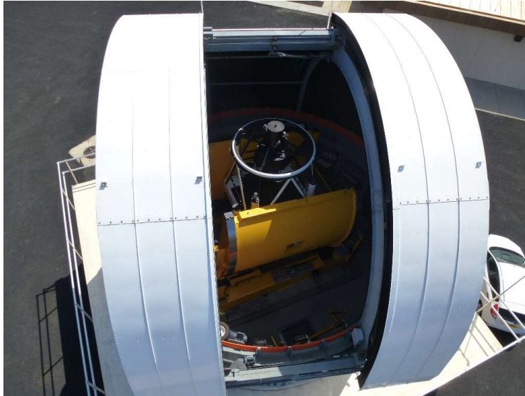
Figure 4. An image of ES-MCAT as seen from the open shutter outside the facility. The 1.3 m telescope is the central white structure inside the yellow double horseshoe mount. The double horseshoe mount allows for rapid transit of the telescope through zenith to allow for constant tracking of resident space objects along any trajectory.
